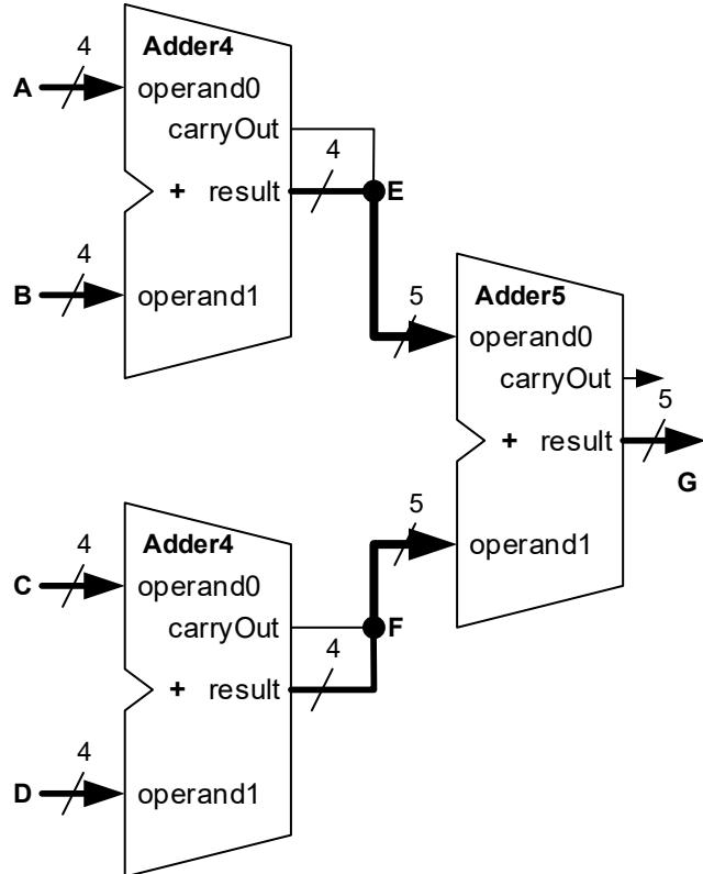
$$\begin{aligned} E &= A + B \text{ (4 + 4 bits = 5 bits)} \\ F &= C + D \text{ (4 + 4 bits = 5 bits)} \\ G &= E + F \text{ (5 + 5 bits = 6 bits)} \end{aligned}$$
