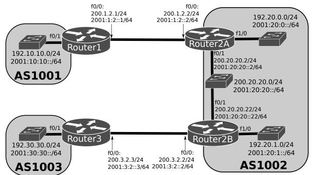
1. Assemble and configure (**only IPv4 addresses**) the above depicted network with three Autonomous Systems (AS). The internal routing protocol in AS1002 is OSPF (<u>network 192.20.0.0/24 is not included</u> <u>in the process</u>). The AS exchange routes using BGP. Using the following commands configure the BGP routing process:
