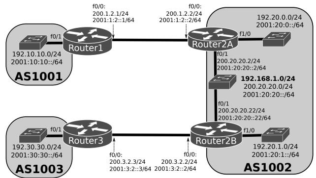
12. To the network assembled and configured before, add an IPv4 private network on AS1002 to the LAN between Router 2A and Router 2B (and include it on OSPFv2 process 1):
