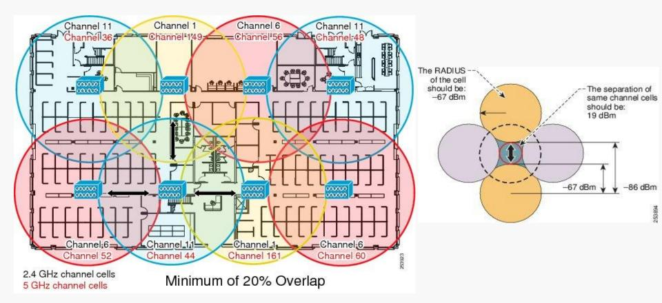
• 802.11n or 802.11ac 5GHz deployment does not have the overlap or collision domain issues of 2.4GHz.
